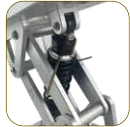
Shock absorber pressure adjustment knob with supplied allen keys
