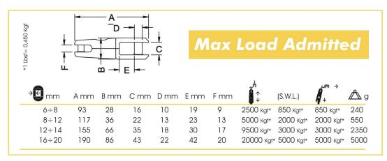
Reminder: The breaking loads of anchor system components must decrease in the following order: A) Deck - B) Bow - roller attachment - C) Chain - D) Anchor connector (see example). By doing so you limit damages and losses in case of failure due to a fouled anchor. It is the obligation of the user to determine whether or not each item is suitable for its intended use.
