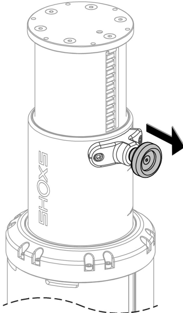
While in a standing position, pull the knob and adjust the seat to the desired height. The pedestal may not rise on its own, depending on the weight of the seat and components installed.
