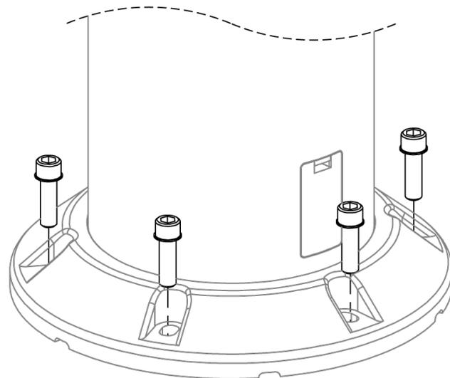
Note: Preferred installation orientation is with the **side access door** of the pedestal facing **aft**.
