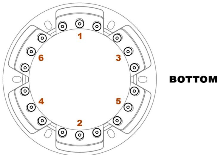
The **mounting flange** of your shock mitigating pedestal is shipped installed in the lowest position available. This torque procedure **must be followed** if loosening the fasteners to adjust the position\* of the mounting flange.
