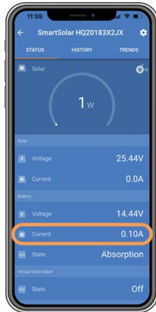
The VictronConnect app shows a close to zero charge current.
