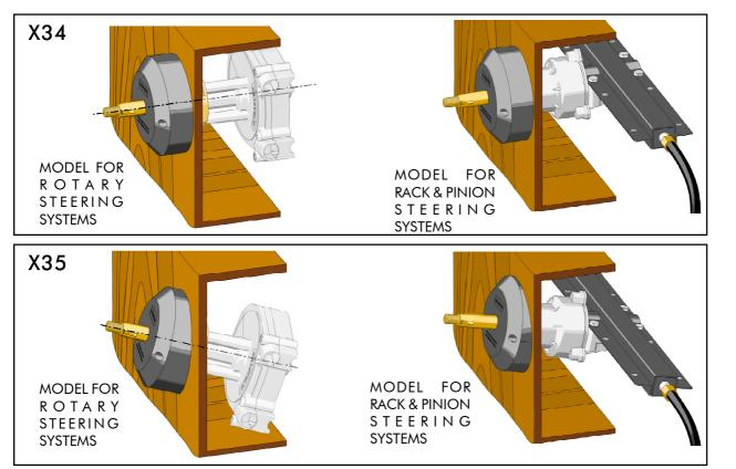
X34 is the 90° mounting bezel. The wheel is perpendicular to the boat dashboard; X35 is the 20° mounting bezel.
