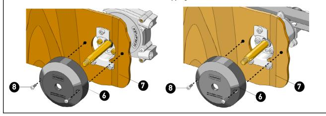
6 Insert the steering wheel (10) on the helm shaft (11) aligning the recess of the hub with the key (9) of the shaft.
