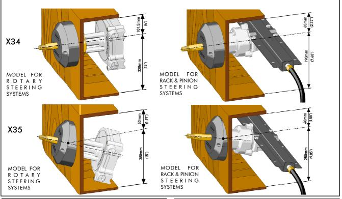
2 By using the supplied drilling template position the steering system in the chosen place and create 3 holes of diameter 10 mm (3/8") and one of diameter 83 mm (3-1/4") in the dashboard.
