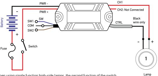
Note: when using single function high-side lamps, the second function of the switch input SW using the brown wire core, is unused. Always refer to the lamp instruction sheet for wiring details.
