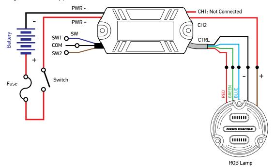
**5B:** RGBW Wiring schematic – only product terminals used are marked:
