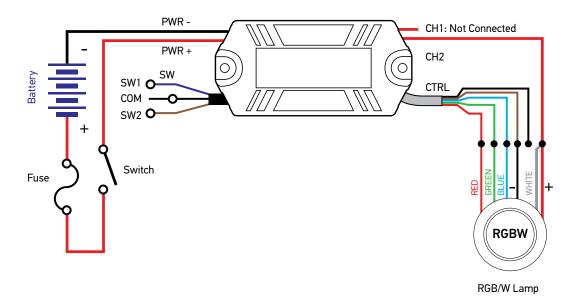
Controller managed with White Light override Wiring schematic – only product terminals used are marked:
