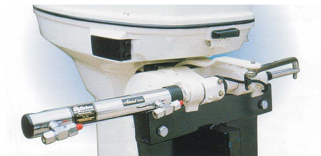
Typical side-mount installation using 210TSE
